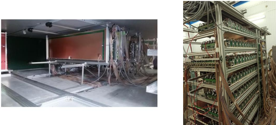
Figure 3.3.2. Left plot: GEM chambers integrated into BM@N experimental setup. Right plot: Cosmic ray test bench.
