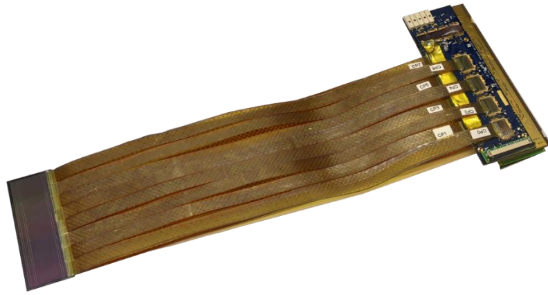
Fig. 3.3.3.3 Photo of the STS module without the shielding foils. The sensor on the left side is connected to the readout electronics on the right side with low-mass micro-cables.
